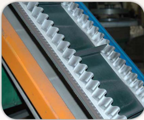
FEZ - 3.2 Industrial chemical conveyor
